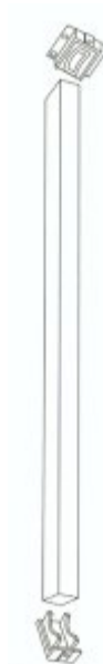
424 Fire exit mullion. 2" x 3" steel tubing round corner, iron construction with iron top and bottom retainers. To be used with two rim type devices on two independent active doors with full double door openings.
