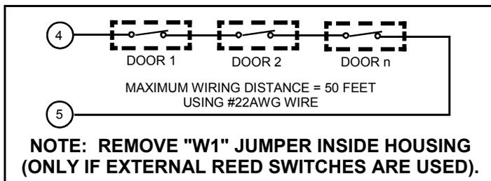
Fig. 2. Multiple door monitoring (wired in series).
